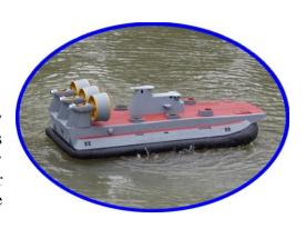
Standing upright at the back of the ship giving the Zubr its distinctive appearance are three ducts housing the 5.5m diameter thrust propellers. The three four-bladed, reversible, variable-pitch air propellers provide the ship with a top speed of 60kt. The vessel has four blowers, model NO-10, fitted with axial fans each 2.5m diameter, two on each side of the vessel to generate the air cushion, the lift air.
