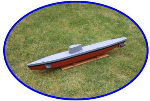
Undine is a submarine originally designed by Hal Harrison and published as a free plan in the October 2001 issue of Marine Modelling International. The plan was for a model that was inexpensive and easy to build requiring only three channels, rudder, front planes and propulsion. The model was 30" long, made from 2mm liteply, designed as a simple dynamic diving submarine with fixed rear planes and controlled by the front planes for depth.
