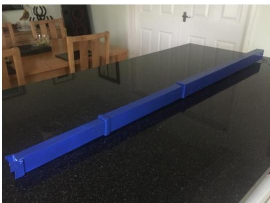
copper tape and micro switches to sense the extremes of travel I eventually placed two of the small motors and gearboxes into the main and second parts, which drove long brass M2 threaded rods in captive M2 threaded bosses. Checking that it all worked as intended I finally sealed the open side of the jib sections and then sprayed the entire extended assembly.
