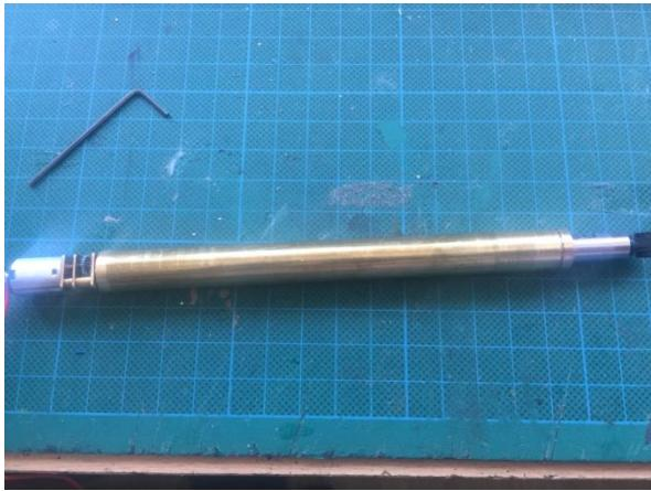
stainless steel threaded rod via an M3 captive nut, force fitted into the lower end of the stainless tube, which acts as the hydraulic piston. This worked well and could extend the tube right out to the end. Since then I have discovered that the huge load imposed on the tiny gearbox caused it to wear away the small bearing under the output shaft.
