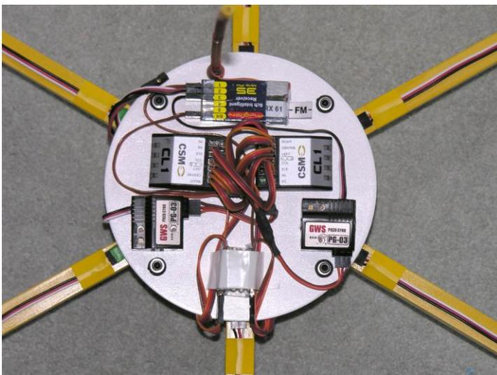
The photo left is a photo of the radio control components, they have been mounted on a separate board which can be moved from model to model, it's painted white. The leads to the ESCs from the mixers have been fed through a hole in the centre of the board in an attempt to keep the assembly reasonably tidy. The radio board is mounted on the airframe using rubber grommets to
