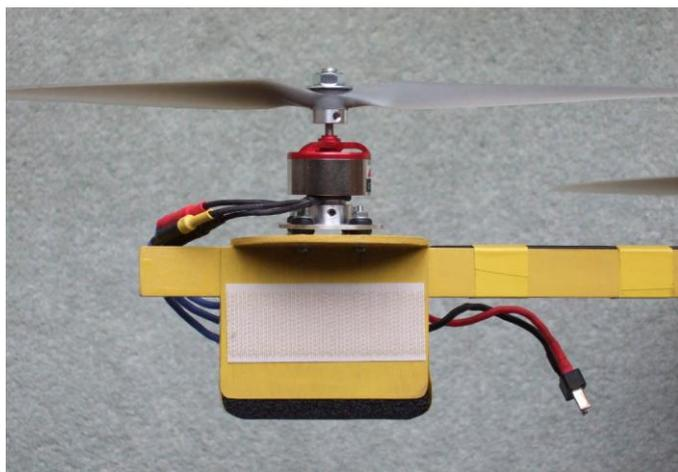
To the left is a photo of one of the arms with its motor, showing the motor mounting arrangement. The Velcro to which the battery is attached can also be seen in this shot, in flight the batteries are secured with elastic bands.
