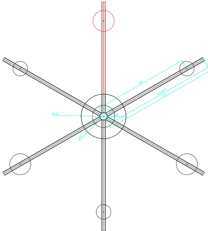
The arms that support the motors for this machine are spaced at 60deg to each other with the motors mounted on a 600mm PCD. As with my previous machines, the Tricopter and Quadcopter, the control system uses standard, “off the shelf” RC components, gyros and mixers, on this machine four gyros and two Cyclock CCPM mixers are used.
