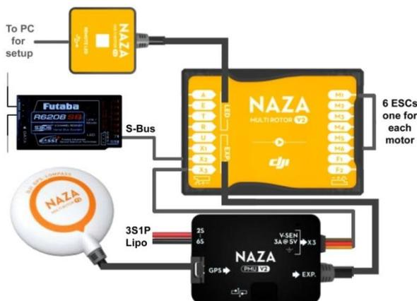
The reworked airframe was populated with the Naza-M control system, the components and their connections are shown to the left. The Naza controller is designed to work with the traditional 1msec – 2msec pulse system (that's the system mostly used for our models), S-Bus or PPM transmissions. S-Bus was chosen because only one lead is required to connect the receiver to the Naza controller. This one lead carries the data for all channels plus the 5volts to power the receiver.
