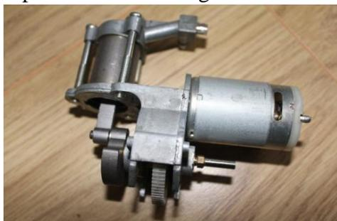
The motor and gearbox used is from a 12volt car tyre pump (left) as it gives the perfect 6:1 reduction needed to power the 6.8cm diameter four bladed brass propeller supplied in the kit. Originally I had intended to remove the the air pump side of the assembly but after experimenting with the smoke generator I discovered that the output of the pump could be utilised to accelerate the smoke on its way up the smoke stack.
