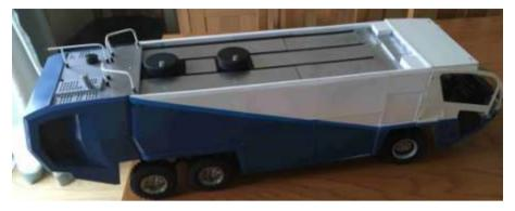
I next began to fabricate the plethora of safety rails using some styrene tube and 16<sup>th</sup> brass rod inserted to give the plastic some rigidity. And then turned my attention to the signage.
