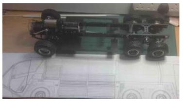
modify the Tamiya chassis so that the measurements were correct. This was achieved by simply moving the entire front axle assembly forward by 1cm.
